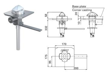
Housing: Steel construction (primed) Locking pin: ø 38 mm (ISO)
