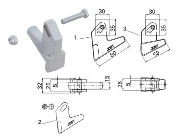
Application: To secure the clamp nuts on twist locks and bolsters to prevent their being released accidentally.
