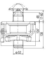
Application: Container chassis/Pitched chassis in frontal position Inner twist lock parts turned 90° For lateral welding to a support or tilt frame rec. gross container weight: max. 34.000 kg Locking pin: ø 52 mm (ISO)
