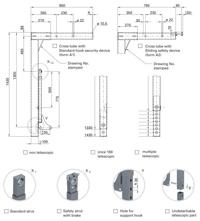
Type definition of a support for swap bodies with a max. weight of up to 18.000 kg
